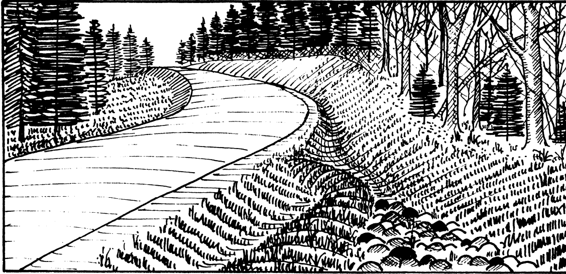
Figure 25. Ditch turnouts channel water away from the road into vegetated buffers.
